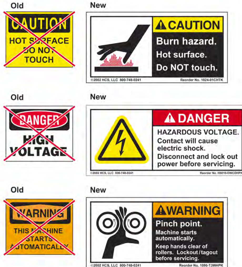
Figure 3. Old and new safety label examples. Note that the new labels are shown in the horizontal format. New labels should convey specific hazard nature, consequence and avoidance information.
